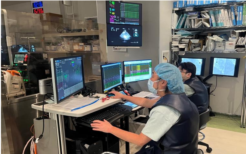
Figure 1. Clinical engineers during catheter ablation. Two CEs operate three-dimensional mapping systems and intracardiac electrogram recording systems to support the procedure. At our institution, we use four types of three-dimensional mapping systems—CARTO 3, EnSite X, OPAL, and AFFERA—and CEs are responsible for operating and managing all of them. One characteristic of CEs in Japan is their ability to support three-dimensional mapping systems from multiple manufacturers and operate each system with an understanding of its specific features. This represents an important area of expertise in arrhythmia care.
